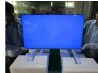
6. Power On Inspection
